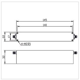
RF Solution offer a wide selection of Band Stop Filter for global customers. BSF-3600M3800A-S is a Band Stop Filter in Rejection Band of 3600~3800 MHz. It is made of high quality materials under a high standard, the Pass Band of this product is DC~3570MHz / 3830~8000MHz, Insertion Loss Max is 2.0 dB and Rejection Min is 45 dB. The component has a good working performance and stability, it is ideal for handling a Rated Power of 10 W.
