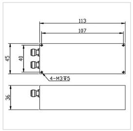
RF Solution offer a wide selection of Band Stop Filter for global customers. BSF-3550M3700A-S is a Band Stop Filter in Rejection Band of 3550~3700 MHz. It is made of high quality materials under a high standard, the Pass Band of this product is DC~3520MHz / 3730~8000MHz, Insertion Loss Max is 3.0 dB and Rejection Min is 80 dB. The component has a good working performance and stability, it is ideal for handling a Rated Power of 20 W.
