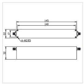
RF Solution offer a wide selection of Band Stop Filter for global customers. BSF-3400M3600A-S is a Band Stop Filter in Rejection Band of 3400~3600 MHz. It is made of high quality materials under a high standard, the Pass Band of this product is DC~3370MHz / 3630~8000MHz, Insertion Loss Max is 2.0 dB and Rejection Min is 45 dB. The component has a good working performance and stability, it is ideal for handling a Rated Power of 10 W.
