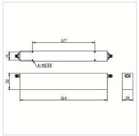
RF Solution offer a wide selection of Band Stop Filter for global customers. BSF-3300M4200A-S is a Band Stop Filter in Rejection Band of 3300~4200 MHz. It is made of high quality materials under a high standard, the Pass Band of this product is DC~3200MHz / 4300~6500MHz, Insertion Loss Max is 2.0 dB and Rejection Min is 70 dB. The component has a good working performance and stability, it is ideal for handling a Rated Power of 20 W.
