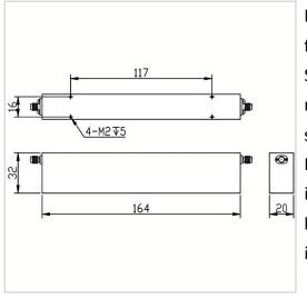
RF Solution offer a wide selection of Band Stop Filter for global customers. BSF-3300M3850A-S is a Band Stop Filter in Rejection Band of 3300~3850 MHz. It is made of high quality materials under a high standard, the Pass Band of this product is DC~3270MHz / 3880~8000MHz, Insertion Loss Max is 3.0 dB and Rejection Min is 40 dB. The component has a good working performance and stability, it is ideal for handling a Rated Power of 20 W.
