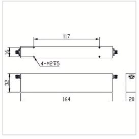
RF Solution offer a wide selection of Band Stop Filter for global customers. BSF-3300M3800A-S is a Band Stop Filter in Rejection Band of 3300~3800 MHz. It is made of high quality materials under a high standard, the Pass Band of this product is DC~3270MHz / 3830~8000MHz, Insertion Loss Max is 3.0 dB and Rejection Min is 40 dB. The component has a good working performance and stability, it is ideal for handling a Rated Power of 20 W.
