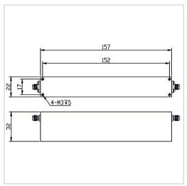
RF Solution offer a wide selection of Band Stop Filter for global customers. BSF-2620M2690A-S is a Band Stop Filter in Rejection Band of 2620~2690 MHz. It is made of high quality materials under a high standard, the Pass Band of this product is DC~2605MHz / 2705~4200MHz, Insertion Loss Max is 2.0 dB and Rejection Min is 40 dB. The component has a good working performance and stability, it is ideal for handling a Rated Power of 20 W.
