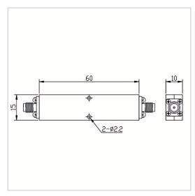
RF Solution offer a wide selection of Band Stop Filter for global customers. BSF-2400M2500A-S is a Band Stop Filter in Rejection Band of 2400~2500 MHz. It is made of high quality materials under a high standard, the Pass Band of this product is DC~2170MHz / 3000~18000MHz, Insertion Loss Max is 2.0 dB and Rejection Min is 50 dB. The component has a good working performance and stability, it is ideal for handling a Rated Power of 10 W.
