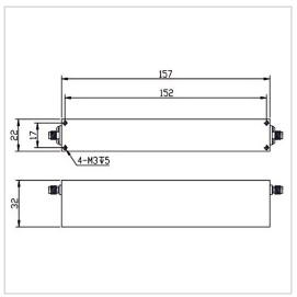
RF Solution offer a wide selection of Band Stop Filter for global customers. BSF-2400M2485A-S is a Band Stop Filter in Rejection Band of 2400~2485 MHz. It is made of high quality materials under a high standard, the Pass Band of this product is DC~2375MHz / 2510~5500MHz, Insertion Loss Max is 2.0 dB and Rejection Min is 40 dB. The component has a good working performance and stability, it is ideal for handling a Rated Power of 10 W.
