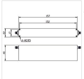
RF Solution offer a wide selection of Band Stop Filter for global customers. BSF-1930M1990A-S is a Band Stop Filter in Rejection Band of 1930~1990 MHz. It is made of high quality materials under a high standard, the Pass Band of this product is DC~1915MHz / 2005~5000MHz, Insertion Loss Max is 2.0 dB and Rejection Min is 40 dB. The component has a good working performance and stability, it is ideal for handling a Rated Power of 20 W.
