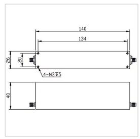
RF Solution offer a wide selection of Band Stop Filter for global customers. BSF-1920M1980A-S is a Band Stop Filter in Rejection Band of 1920~1980 MHz. It is made of high quality materials under a high standard, the Pass Band of this product is DC~1900MHz / 2010~3000MHz, Insertion Loss Max is 2.0 dB and Rejection Min is 30 dB. The component has a good working performance and stability, it is ideal for handling a Rated Power of 10 W.
