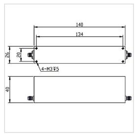
RF Solution offer a wide selection of Band Stop Filter for global customers. BSF-1880M1920A-S is a Band Stop Filter in Rejection Band of 1880~1920 MHz. It is made of high quality materials under a high standard, the Pass Band of this product is DC~1865MHz / 1935~3000MHz, Insertion Loss Max is 2.0 dB and Rejection Min is 40 dB. The component has a good working performance and stability, it is ideal for handling a Rated Power of 10 W.
