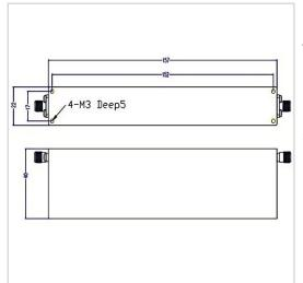
RF Solution offer a wide selection of Band Stop Filter for global customers. BSF-1805M1880A-S is a Band Stop Filter in Rejection Band of 1805~1880 MHz. It is made of high quality materials under a high standard, the Pass Band of this product is DC~1785MHz / 1900~6000MHz, Insertion Loss Max is 2.0 dB and Rejection Min is 60 dB. The component has a good working performance and stability, it is ideal for handling a Rated Power of 30 W.
