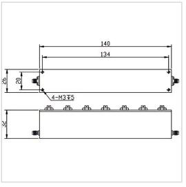
RF Solution offer a wide selection of Band Stop Filter for global customers. BSF-1800M2000A-S is a Band Stop Filter in Rejection Band of 1800~2000 MHz. It is made of high quality materials under a high standard, the Pass Band of this product is DC~1750MHz / 2050~3000MHz, Insertion Loss Max is 2.0 dB and Rejection Min is 40 dB. The component has a good working performance and stability, it is ideal for handling a Rated Power of 30 W.
