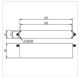
RF Solution offer a wide selection of Band Stop Filter for global customers. BSF-1710M1780A-S is a Band Stop Filter in Rejection Band of 1710~1780 MHz. It is made of high quality materials under a high standard, the Pass Band of this product is DC~1695MHz / 1795~3000MHz, Insertion Loss Max is 2.0 dB and Rejection Min is 40 dB. The component has a good working performance and stability, it is ideal for handling a Rated Power of 10 W.
