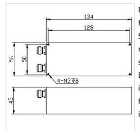
RF Solution offer a wide selection of Band Stop Filter for global customers. BSF-1695M1710A-N is a Band Stop Filter in Rejection Band of 1495~1710 MHz. It is made of high quality materials under a high standard, the Pass Band of this product is DC~1685MHz / 1720~5000MHz, Insertion Loss Max is 2.5 dB and Rejection Min is 80 dB. The component has a good working performance and stability, it is ideal for handling a Rated Power of 10 W.
