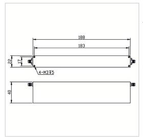
RF Solution offer a wide selection of Band Stop Filter for global customers. BSF-1400M1600A-S is a Band Stop Filter in Rejection Band of 1400~1600 MHz. It is made of high quality materials under a high standard, the Pass Band of this product is DC~1340MHz / 1660~5000MHz, Insertion Loss Max is 1.5 dB and Rejection Min is 60 dB. The component has a good working performance and stability, it is ideal for handling a Rated Power of 20 W.
