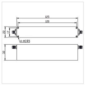
RF Solution offer a wide selection of Band Stop Filter for global customers. BPF-2500M2570A-S is a Band Stop Filter in Rejection Band of 2500~2570 MHz. It is made of high quality materials under a high standard, the Pass Band of this product is DC~2170MHz / 3000~18000MHz, Insertion Loss Max is 3.0 dB and Rejection Min is 40 dB. The component has a good working performance and stability, it is ideal for handling a Rated Power of 10 W.
