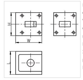
RF Solution offer a wide selection of Waveguide Circulator for global customers. BH8911-WR187 is a Waveguide Circulator in Frequency Range of 4.0~6.0 GHz. It is made of high quality materials under a high standard, the Bandwidth Max of this product is 10%, Insertion Loss Max is 0.30 dB and Isolation Min is 23.0 dB. The component has a good working performance and stability, it is ideal for handling a Forward Power of /.
