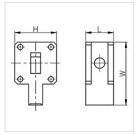
RF Solution offer a wide selection of Waveguide Isolator for global customers. BG8920-WR187 is a Waveguide Isolator in Frequency Range of 8.0~12.0 GHz. It is made of high quality materials under a high standard, the Bandwidth Max of this product is 10%/20%, Insertion Loss Max is 0.25~0.30 dB and Isolation Min is 20.0~23.0 dB. The component has a good working performance and stability, it is ideal for handling a Forward Power of /.
