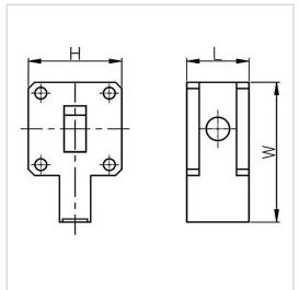
RF Solution offer a wide selection of Waveguide Isolator for global customers. BG6816-WR137 is a Waveguide Isolator in Frequency Range of 5.4~8.0 GHz. It is made of high quality materials under a high standard, the Bandwidth Max of this product is 20%, Insertion Loss Max is 0.30 dB and Isolation Min is 23.0 dB. The component has a good working performance and stability, it is ideal for handling a Forward Power of /.
