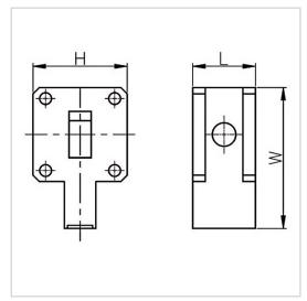
RF Solution offer a wide selection of Waveguide Isolator for global customers. BG5010-WR137 is a Waveguide Isolator in Frequency Range of 6.8~7.5 GHz. It is made of high quality materials under a high standard, the Bandwidth Max of this product is 20%, Insertion Loss Max is 0.30 dB and Isolation Min is 20.0 dB. The component has a good working performance and stability, it is ideal for handling a Forward Power of /.
