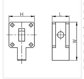
RF Solution offer a wide selection of Waveguide Isolator for global customers. BG3676-WR112 is a Waveguide Isolator in Frequency Range of 7.0~10.0 GHz. It is made of high quality materials under a high standard, the Bandwidth Max of this product is 10%, Insertion Loss Max is 0.25~0.30 dB and Isolation Min is 23.0~25.0 dB. The component has a good working performance and stability, it is ideal for handling a Forward Power of /.
