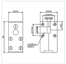
RF Solution offer a wide selection of Waveguide Isolator for global customers. BG3070-WR22 is a Waveguide Isolator in Frequency Range of 43.0~46.0 GHz. It is made of high quality materials under a high standard, the Bandwidth Max of this product is 100%, Insertion Loss Max is 0.25 dB and Isolation Min is 18.0 dB. The component has a good working performance and stability, it is ideal for handling a Forward Power of /.
