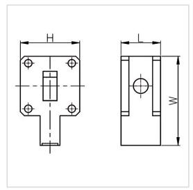
RF Solution offer a wide selection of Waveguide Isolator for global customers. BG2851-WR90 is a Waveguide Isolator in Frequency Range of 8.0~12.4 GHz. It is made of high quality materials under a high standard, the Bandwidth Max of this product is 5%, Insertion Loss Max is 0.30~0.40 dB and Isolation Min is 20.0~23.0 dB. The component has a good working performance and stability, it is ideal for handling a Forward Power of /.
