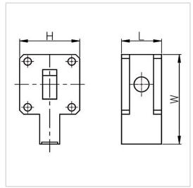
RF Solution offer a wide selection of Waveguide Isolator for global customers. BG1348-WR90 is a Waveguide Isolator in Frequency Range of  $8.0\sim12.4$  GHz. It is made of high quality materials under a high standard, the Bandwidth Max of this product is 200M/300M, Insertion Loss Max is  $0.30\sim0.40$  dB and Isolation Min is  $23.0\sim25.0$  dB. The component has a good working performance and stability, it is ideal for handling a Forward Power of /.
